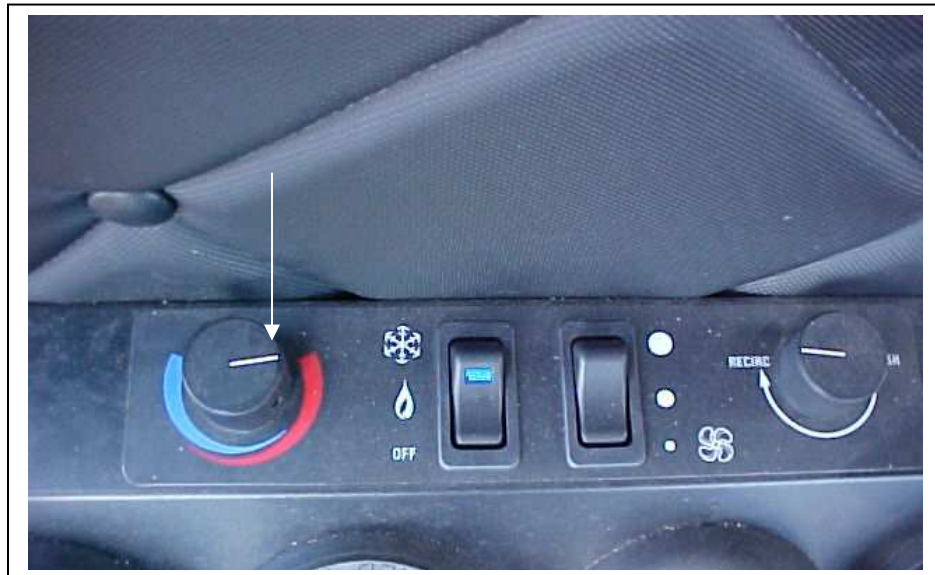
Figure 2 – Upper Cab Air Conditioner/Heater Control Panel
