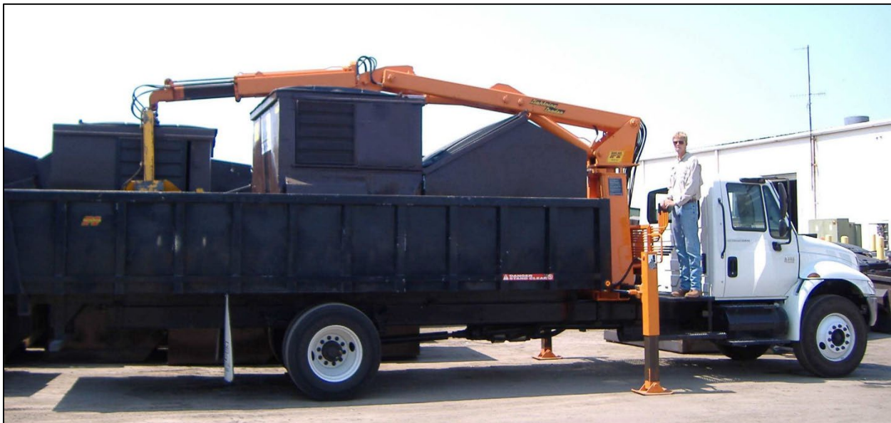
Place any taller containers in the center of the body to allow the lowest possible boom height.
