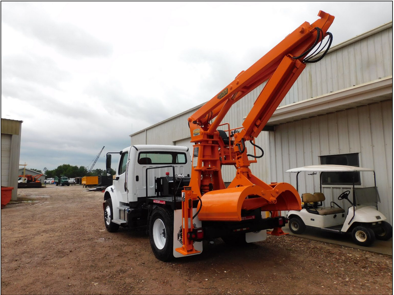
Stowing the bucket for transport when NOT towing a trailer.
