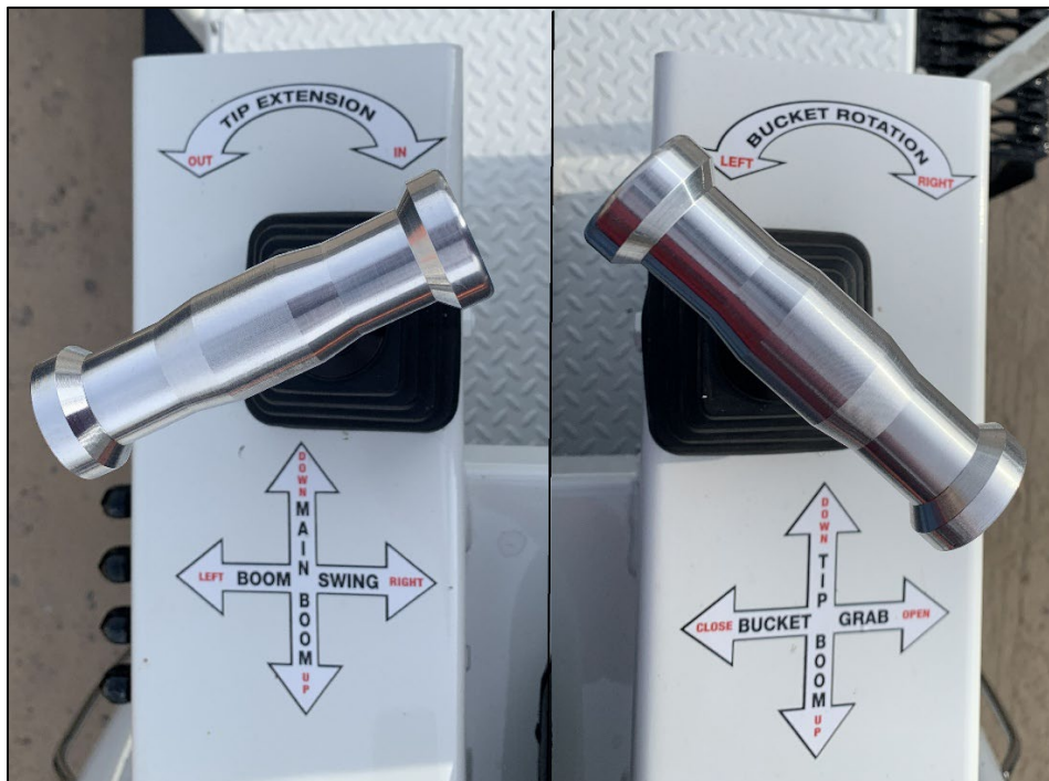
Top-Seat Joystick Control Functions
