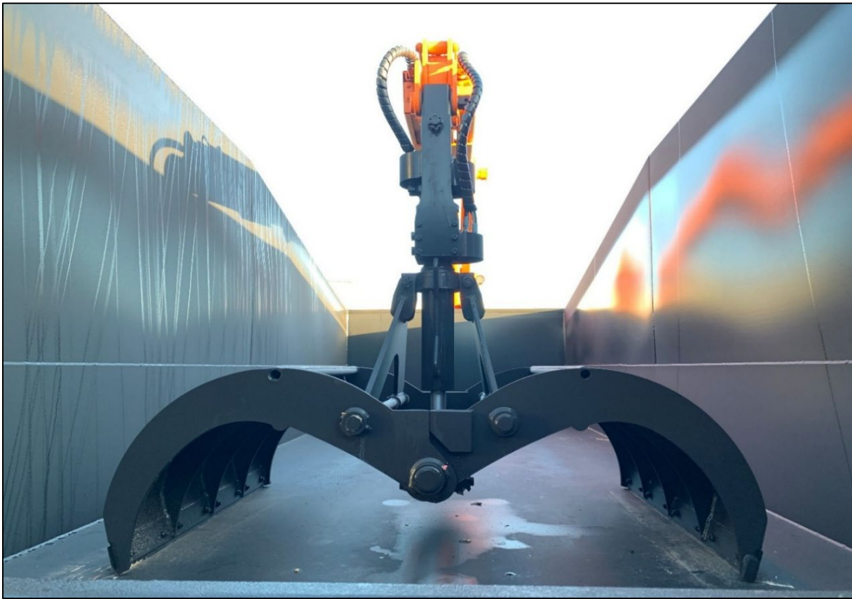
When the boom is stowed, the bucket sides should be parallel to the sides of the dump body.
