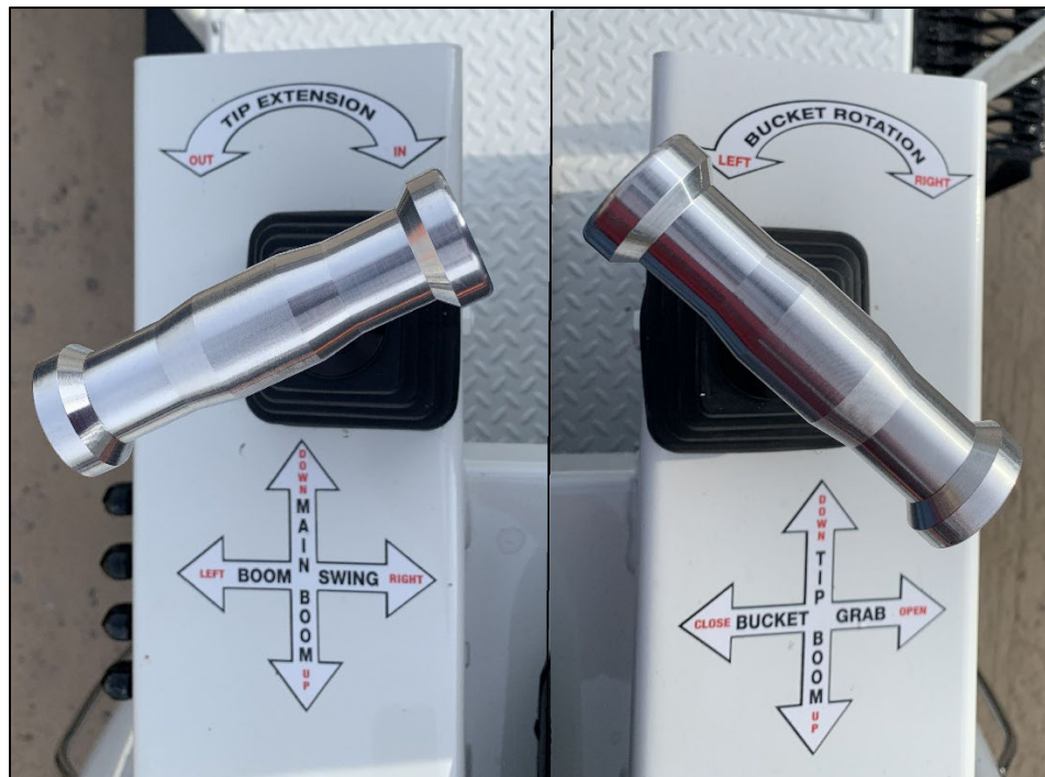
Top-Seat joystick control functions
