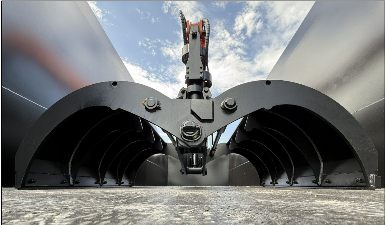
When the boom is stowed, the bucket sides should be parallel to the sides of the dump body.
